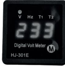
(V) - this mode displays the voltage level of the generator in volts
